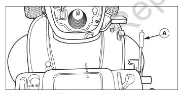
Figure 12. Mower Cutting Height Adjustment A. Adjustment Lever
